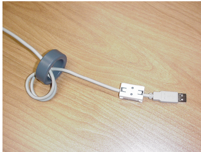
Figure 11 - Example of a USB Cable Using Ferrites
